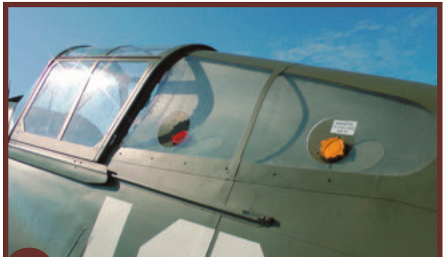
A bright red gasoline cap and a bright yellow oil cap—both tanks accessed through the P-40C’s aft cockpit glazing—were faithfully restored on AK295.
