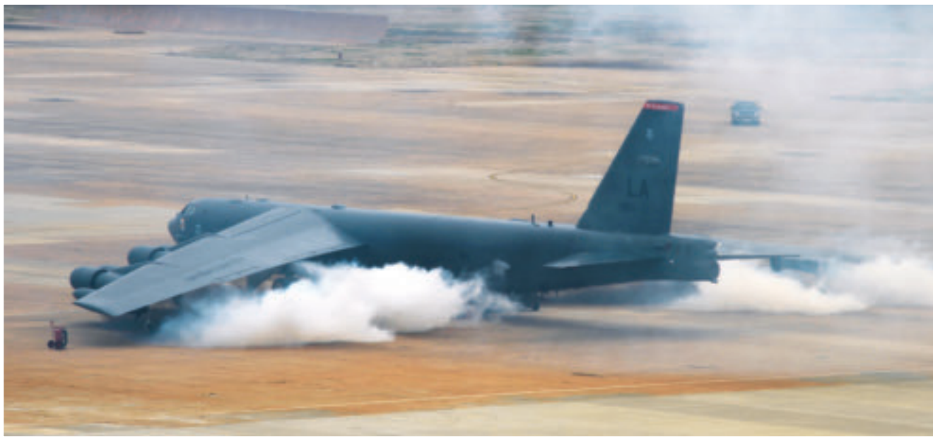
Boom Shaka Laka: A B-52H gets a starting boost from starter cartridges during a minimum interval aircraft takeoff exercise at Barksdale AFB, La. B-52 crews use the “cart start” maneuver to get the bird in the air as fast as possible. Eight starter cartridges filled with gunpowder—one per engine—explode, jump-starting the engines faster than a normal takeoff does.
